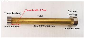
Make a pencil mark 8.7mm from end. Use a parting tool to cut a 8.7mm tenon down to the diameter of the bushing( Diameter: 10.4mm). Make sure you keep a sharp outside 90° corner on the tenon.
