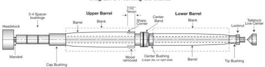
Diagram B / Turning the Blanks
