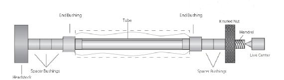
Diagram B - Turning the Blank
